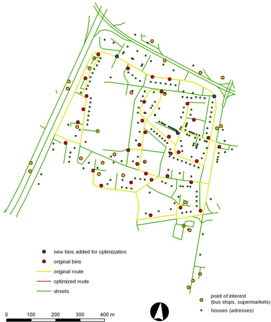
Fig. 5 Original (yellow) and optimized (red) route vehicles for collection of separated waste. The blue points show new added (containers) bins for spatial optimization.
